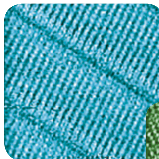
Gold on mica. Island dimensions and step heights can be measured with traxSTM Scan size: 10 \mu\text{m}
